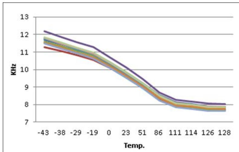
Figure 31-3 LIRC deviation under V<sub>DD</sub> = 2.4 V
