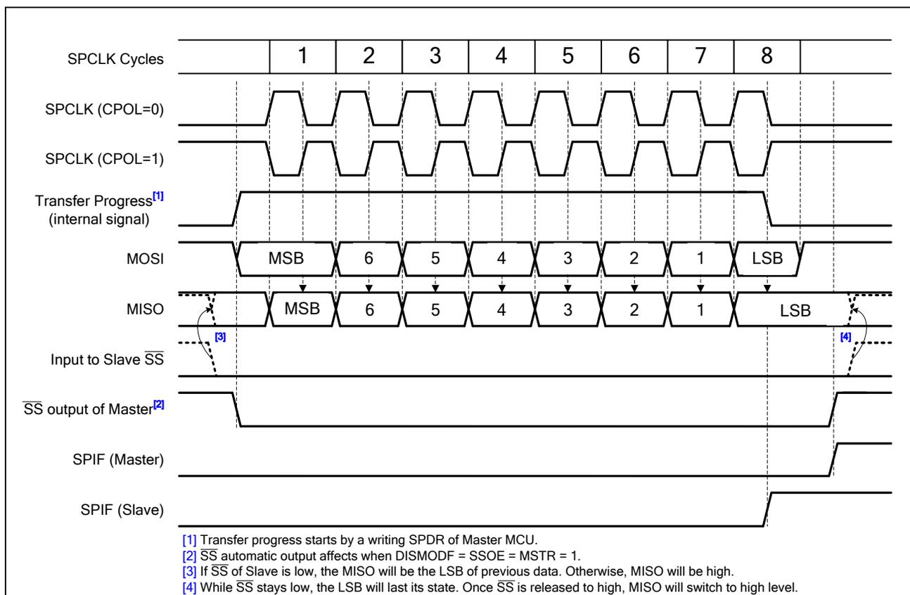
Figure 14-6. SPI Clock and Data Format with CPHA = 1
