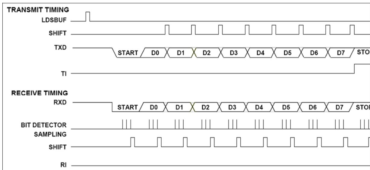
Figure 13-2. Serial Port Mode 1 Timing Diagram
