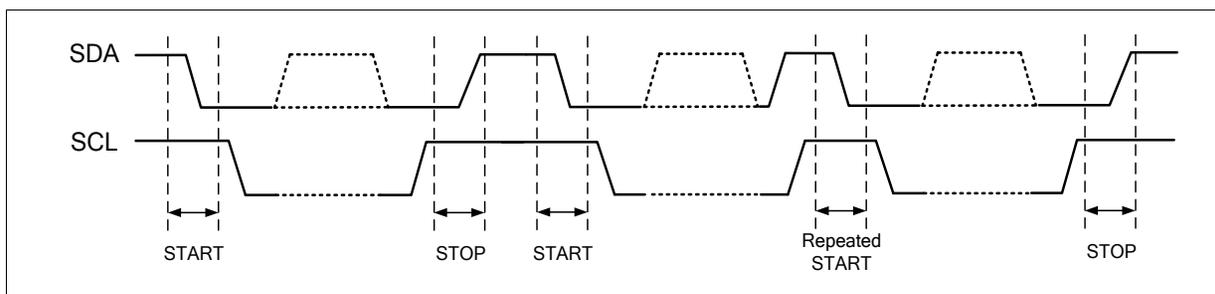
Figure 15-3. START, Repeated START, and STOP Conditions
