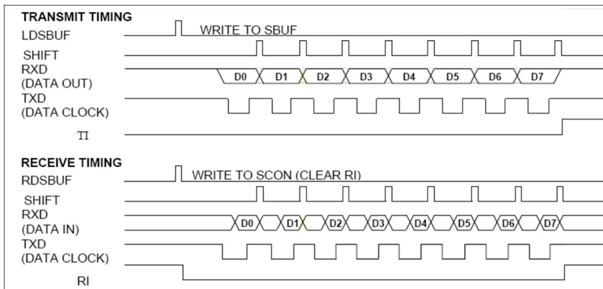
**Figure 13-1. Serial Port Mode 0 Timing Diagram**
