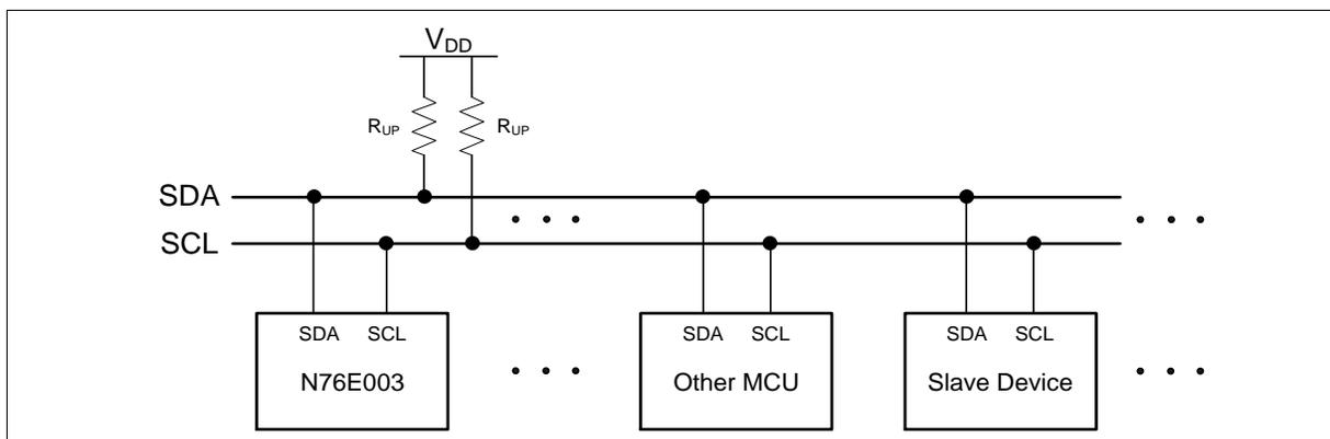
Figure 15-1. I<sup>2</sup>C Bus Interconnection
