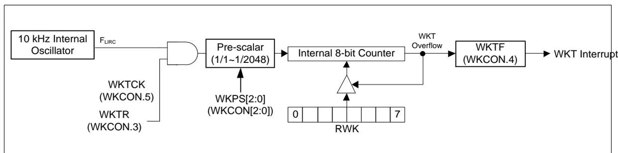
Figure 12-1. Self Wake Up Timer Block Diagram
