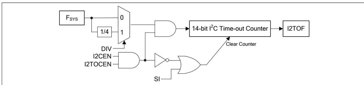
Figure 15-12. I<sup>2</sup>C Time-Out Counter
