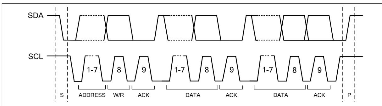
Figure 15-4. Data Format of One I<sup>2</sup>C Transfer
