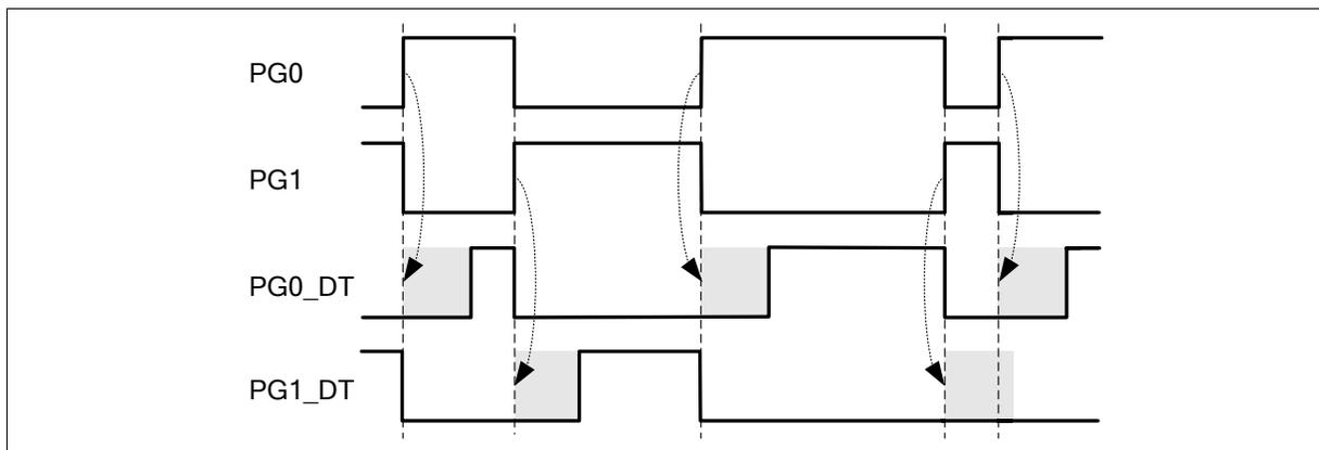
Figure 17-5. PWM Complementary Mode with Dead-time Insertion
