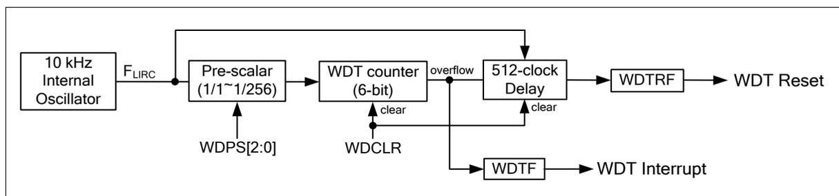
Figure 11-1. WDT as A Time-Out Reset Timer
