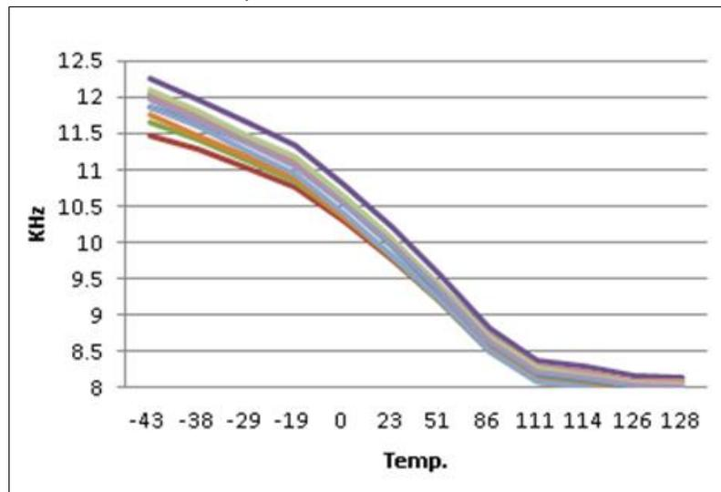
Figure 31-2 LIRC deviation under V<sub>DD</sub> = 5.5 V
