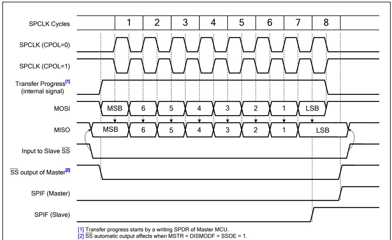
Figure 14-5. SPI Clock and Data Format with CPHA = 0
